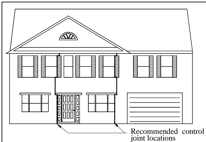
Figure 2—Example of Residential Control Joint Placement
